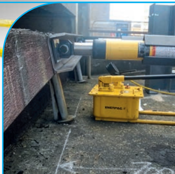
Mobile on-site hydraulic ram test on existing barrier
