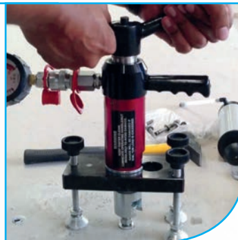
Mobile on-site fixings pull out test
